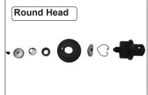
The head can be opened up to access the ratchet mechanism either by releasing the circlip using a pair of internal circlip pliers (fig.1) or removing the securing screws (figs. 2,3 & 4).
