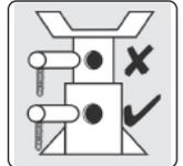
Fit pin through both the stand collar and the centre tube
