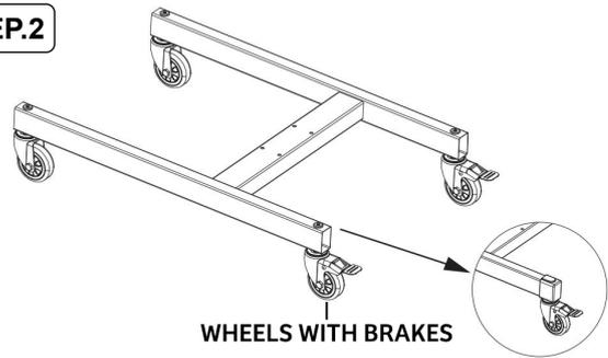
2. Pass the tube nut through the square tube hole of the underframe. Fit the 3" wheels, and tighten with a wrench. Ensure the wheels with brakes are installed at the correct end of the underframe. Insert the plugs back onto the underframe.
