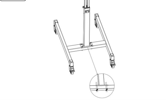
3. Place the support frame assembly on the base as shown, paying attention to the front and rear orientation. Secure with bolt, flat washer and anti-loose nut, using the wrench provided.
