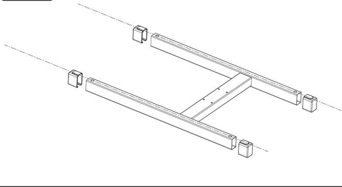
1. Remove the plugs from both sides of the underframe. Leave them off until the wheels have been installed.
