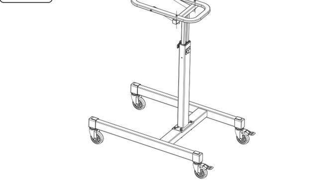
5. Install the upper support tube assembly on the support frame assembly as shown. Secure with 2 hexagonal screws, flat washers and anti-loose nuts, using the wrench provided.
