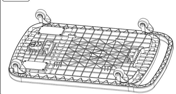
6. Install the 2" wheels in the screw holes of the tool tray as shown. Tighten with the wrench provided.
