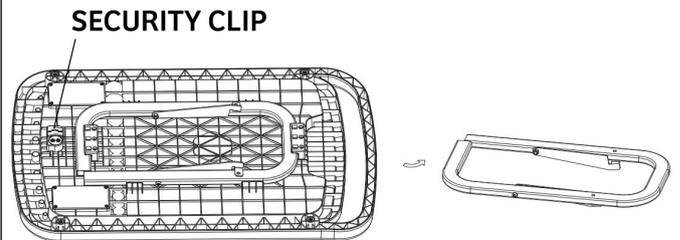
4. Ensure the security clip is 'open' as shown above. Push the upper support frame assembly horizontally to the left and remove it from the tool tray assembly.
