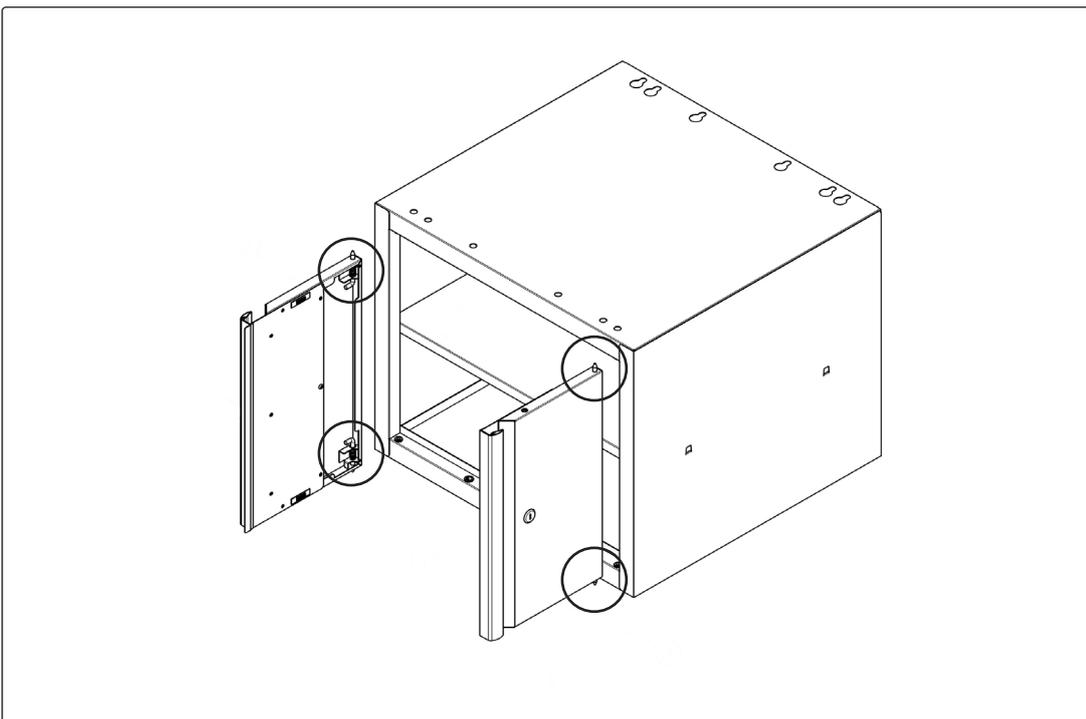
Step 2. Attach Cabinet Door Right 3, and Left Side 2 to Cabinet Body 1 using the spring loaded catches on door. See Illustration.
