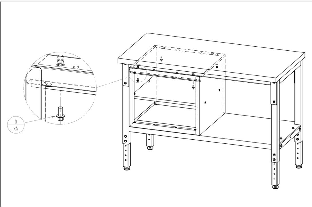
Step 1. Attach Cabinet Body (1) to the bench using supplied hardware. See illustration.
