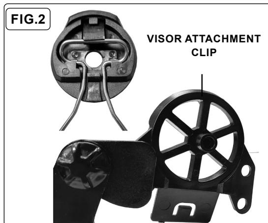
2. Reassemble using the visor attachment clip.
